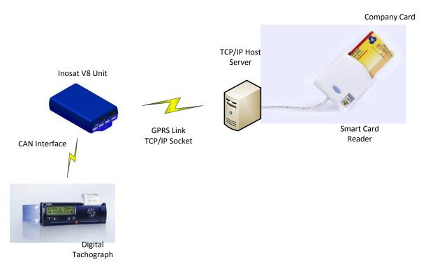
As illustrated by the above drawing, it is possible to tachograph data from remote vehicles, without needing to access directly to the VU (Vehicle Unit).
